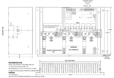
Note: SAFETY WARNING - Metal parts, in particular the heatsink, may get very hot when the unit is fully operational.
