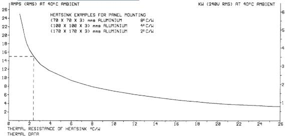
WITH HEATSINK AS SPECIFIED, THE MAXIMUM LOAD CURRENT CAN BE DETERMINED. THIS IS THE MAXIMUM LOAD CURRENT POSSIBLE WITHOUT EXCEEDING THE DEVICE RATINGS.
