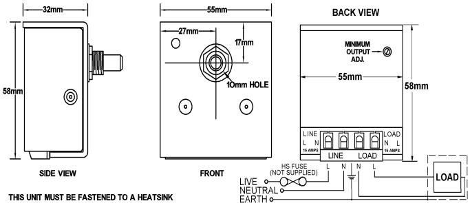
RATED AT 2 °C/W FOR 15A OPERATION. **HEATSINK PASTE ESSENTIAL** FOR GOOD THERMAL CONTACT.
