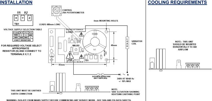
NOTE: REMOTE POTENTIOMETER LEADS ARE AT HAZARDOUS LIVE POTENTIAL AND OTHER COMPONENTS ARE, OR IN FAULT CONDITIONS MAY BECOME HAZARDOUS LIVE.
