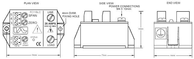
USE HEATSINK COMPOUND FOR EFFECTIVE THERMAL COUPLING WARNING LIVE TERMINALS
