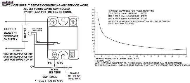
**PROTECTION NOTE**: Use a minimum 3A Rated Cable for the +VE supply of the DCM controller for controller protection a 'TRANSIL' component device is recommended to be fitted (hard wired) across the following supply terminals – "M3 +ve" and "M5 – ve IN".
