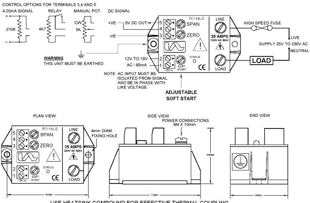
USE HEATSINK COMPOUND FOR EFFECTIVE THERMAL COUPLING WARNING LIVE TERMINALS SWITCH OFF MAINS SUPPLY BEFORE COMMENCING ANY SERVICE WORK
