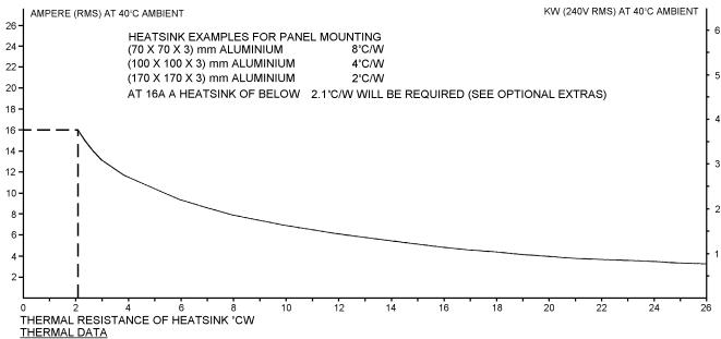
WITH HEATSINK AS SPECIFIED, THE MAXIMUM LOAD CURRENT CAN BE DETERMINED. THIS IS THE MAXIMUM LOAD CURRENT POSSIBLE WITHOUT EXCEEDING THE DEVICE RATING.
