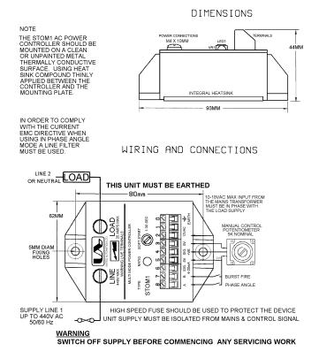
CONTROL OPTIONS DC INPUT VOLTAGE CONTROL TERMINALS 3,4 AND 5 □ 3 = 0V 🔲 4 = 0 TO 5V □ 5 = 5V OUTPUT 5K INPUT CURRENT CONTROL TERMINALS 3 AND 6 □ 3 = 0V □ 6 = 4-20mA 240R INPUT MODE A PHASE ANGLE TERMINAL A AND 5 🔲 A = 5V □ 5 = 5V MODE B BURST FIRE TERMINALS B AND 5 ☐ B = 5V ☐ 5 = 5V MODE A AND B START IN PHASE ANGLE SWITCHING TO BURST FIRE TERMINAL A,B AND 5 🗆 A = 5V 🛛 B = 5V □ 5 = 5V PHASE REFERENCE AND SUPPLY TERMINALS 1 AND 2 10V TO 18V AC AT 75 mA
