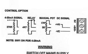
SWITCH OFF MAINS SUPPLY BEFORE COMMENCING ANY SERVICING WORK
