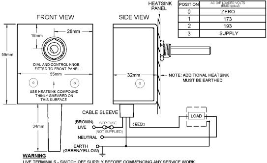
LIVE TERMINALS - SWITCH OFF SUPPLY BEFORE COMMENCING ANY SERVICE WORK. FOR HEATSINK PANEL MOUNTING
