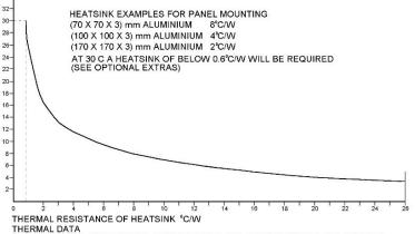
WITH HEATSINK AS SPECIFIED, THE MAXIMUM LOAD CURRENT CAN BE DETERMINED. THIS IS THE MAXIMUM LOAD CURRENT POSSIBLE WITHOUT EXCEEDING THE DEVICE RATING
