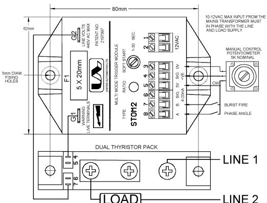
**CONTROL OPTIONS** DC INPUT VOLTAGE CONTROL TERMINALS 3,4 AND 5 □ 3 = 0V ☐ 4 = 0 TO 5V ☐ 5 = 5V OUTPUT ☐ 5K INPUT
