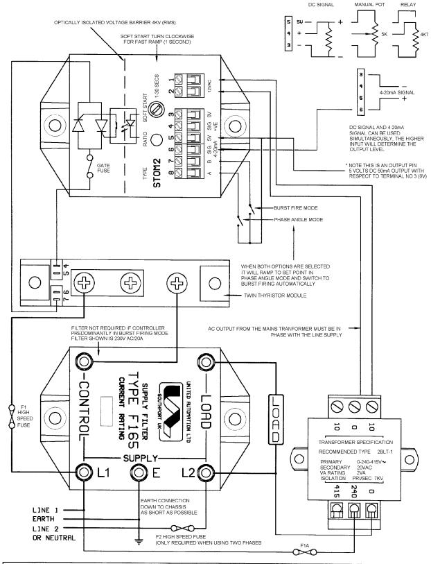
MATCH MAINS SUPPLY FILTER TO THE SUPPLY VOLTAGE AND MAX. LOAD CURRENT IN ORDER TO COMPLY WITH BSEN 550081-2 WHEN USED IN PHASE ANGLE MODE
