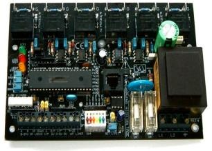
most inductive loads via thyristor pairs on three phase assemblies. SCR Power handling gives smooth proportional control to all types of industrial processes which include furnaces, electroplating, controlled rectifiers and transformers.
