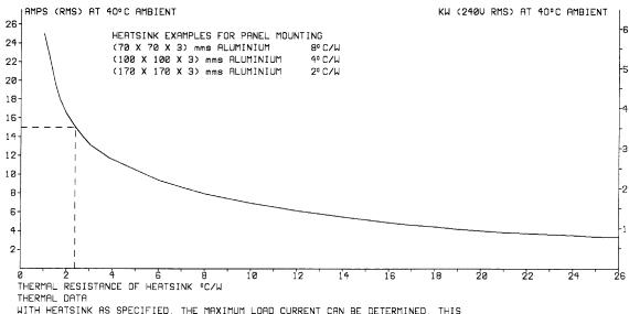
WITH HEATSINK AS SPECIFIED, THE MAXIMUM LOAD CURRENT CAN BE DETERMINED. THIS IS THE MAXIMUM LOAD CURRENT POSSIBLE WITHOUT EXCEEDING THE DEVICE RATINGS.
