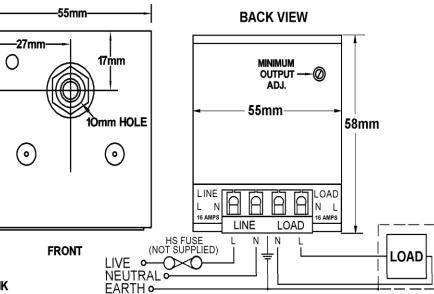
THIS UNIT MUST BE FASTENED TO A HEATSINK RATED AT 2  $^{\circ}$ C/W FOR 15A OPERATION. HEATSINK PASTE ESSENTIAL FOR GOOD THERMAL CONTACT.
