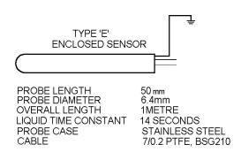
NOTE: Good thermal bonding of sensor is required, where appropriate, to ensure controller performance reaction time, i.e. for thermal bonding of sensor to metal heatsink, it is recommended that heatsink paste is used.
